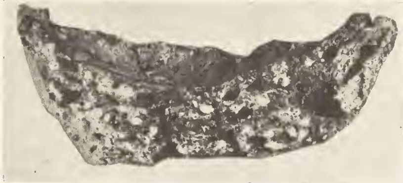
1. Side view of the Horsham natural slag specimen, showing saucer-shape and vesicular character of the interior. (Natural size.)
